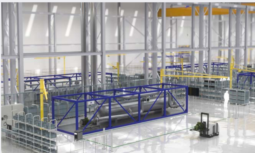
Rolls-Royce SMR factories will produce hundreds of prefabricated and pre-tested modules ready for assembly on site into a complete nuclear power plant. Image: Rolls-Royce SMR.
