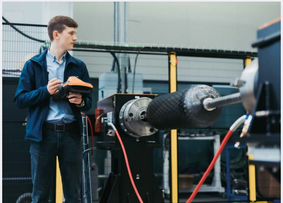
The AMRC is using filament winding technology to manufacture lower cost and lightweight composite pressure vessels that can store hydrogen to be used as a clean energy source.
