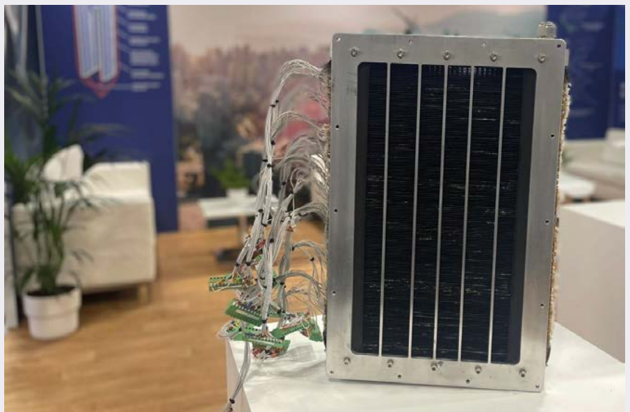
ZeroAvia's fuel cell stack that will be used to develop rate capable assemblies for, with the completed stacks aimed to go into its 2000 powertrain aircraft. Image: ZeroAvia.
