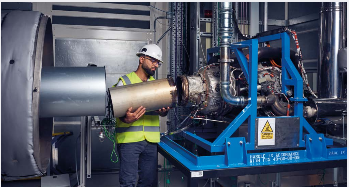
Ihab Ahmed, researcher, setting up an auxiliary power unit testing rig at the TERC facility.
