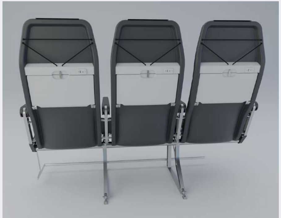
A render of the new, lighter weight seat design developed by AMRC engineers. Image: Mirus Aircraft Seating.
