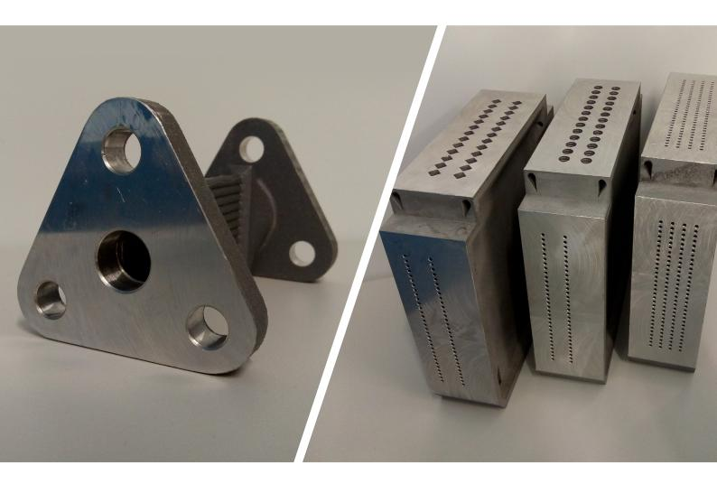
All components were additively manufactured on a Renishaw AM400HT unit, with subsequent post processing including stress-relieving heat treatment and face milling to produce a sealing face suitable for the testing equipment at Meggitt.
