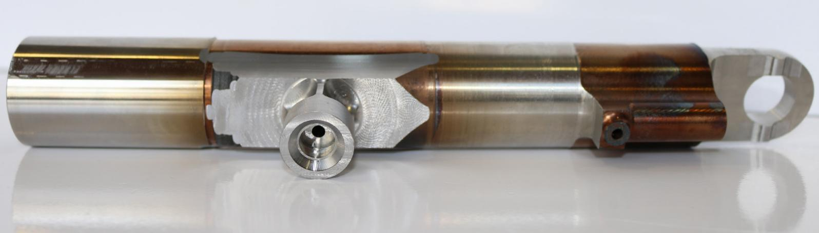
The current production route for this aircraft engine component uses a solid bar feedstock, but using hybrid manufacturing the stock material can be changed to a tube material. Additive and subtractive processes can be optimally sequenced so that stock is added on the tube, increasing the stability of the machining operations and generating the final required geometry.
