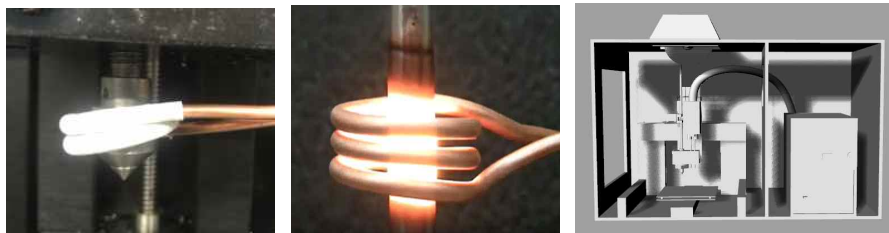
<Fig .1 Conceptual drawing of additive manufacturing process for direct melting extrusion of metal wire by induction heating>
