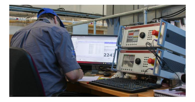
The ASTC has the ability to control tests of up to 8 loading points via MOOG control systems portable test controllers. Tests can be conducted in load or displacement control. 'Real world' data can be transferred into test programmes and accelerated fatigue tests or multi-load strength testing can easily be carried out at the ASTC.
