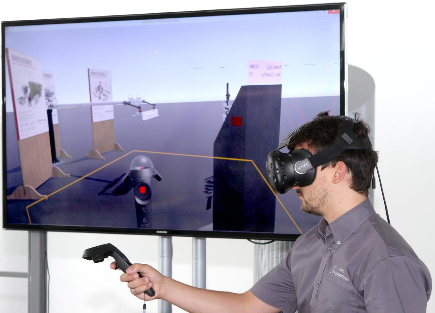
“The simulations allow engineers to customise fixturing tooling and adapt them to the press shop environment in the pre-production stages to allow design revisions before physical models are built.” **Michael Lewis.**
