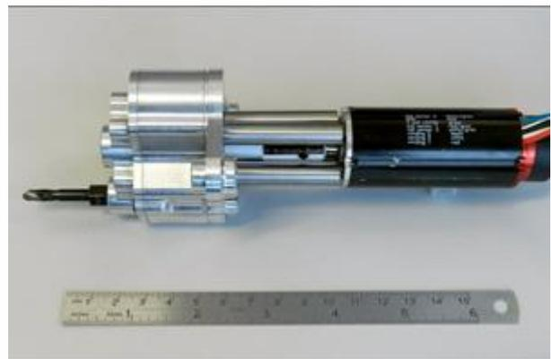
"Our solution was what we have called a passive input gearbox, which automatically changes gear ratios depending on the rotation direction of the drive motor, while always maintaining the same drill rotation direction," says Nicholson.
