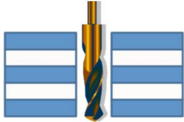
These composite and metallic materials have very different material properties, and would normally require different drilling parameters. For example, drilling a carbon fibre composite commonly requires high speed and low torque, while drilling titanium typically requires low speed and high torque. Drilling a hole through a stack of both materials demands a tool which can quickly and efficiently switch between these two modes.
