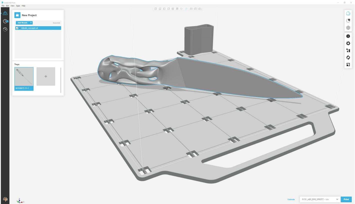
A GrabCAD print setup up of a concept knife model. At this stage the build orientation, supports and scan strategy is defined. Once the correct parameters are determined the knife is sliced and sent to a Fused Deposition Modelling (FDM) machine to be printed in polymer. Once 3D printed, this allows the designer to visualise the end concept cost effectively before moving onto metallic prototyping.
