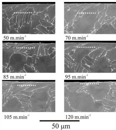
Figure 2 Electron backscatter images of the machined surface with increasing surface speed. The delineated line signifies the interface between the undeformed bulk material and the average depth of deformation assessed using beta
