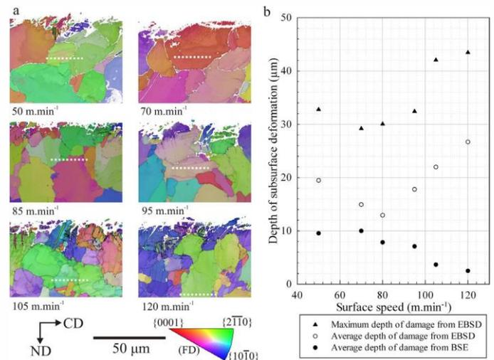
Figure 3 (a) EBSD inverse pole figure (IPF) maps of the machined surface with increasing surface speed. The white delineated line signifies the interface between the undeformed bulk material and the maximum depth of damage. (b) Graph illustrating the effect of surface speed on the depth of surface deformation assessed by measuring beta distortion using backscatter electron images and EBSD.
