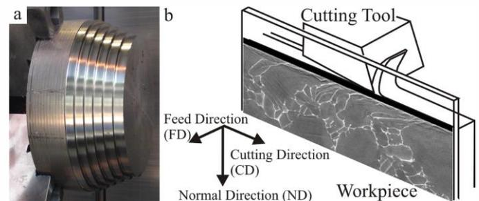
Figure 1 a) Photograph of stepped Ti-834 billet workpiece prior to the outer diameter precision turning trials; b) Schematic illustrating the cutting process and typical subsurface microstructure deformation, sectioned parallel to the cutting direction.
