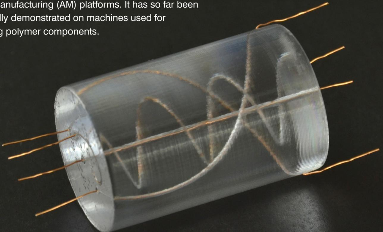
AMRC Development Engineer and AM specialist Mark Cocking, developed the new technique, he said: “The technology has scope to simultaneously add multiple, industry recognised threads of differing materials into one component to give that component additional functions. This will open AM up to a greater variety of uses.”
